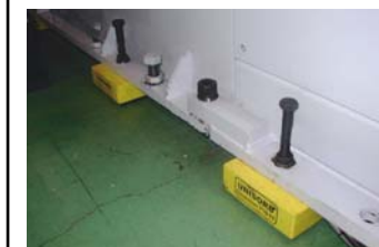
Leveling pad for installation
